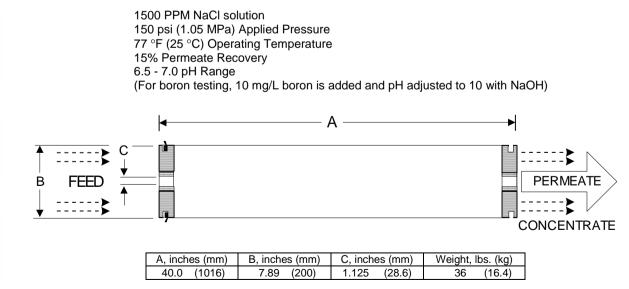
Notice: Permeate flow for individual elements may vary + or - 15 percent. Membrane active area may vary +/-4%. All membrane elements are supplied with a brine seal, interconnector, and o-rings. Elements are enclosed in a sealed polyethylene bag containing less than 1.0% sodium meta-bisulfite solution, and then packaged in a cardboard box.
