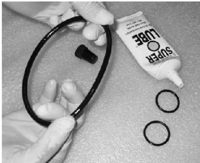
Lubricating Plug seals and O-rings
