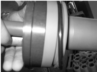
Removal of the Plug Seal
