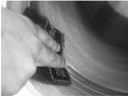
Cleaning inside the vessel
