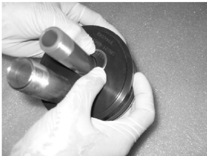
Removal of the Circlip
