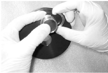
Installing of F/C Port & Port Retainer set
