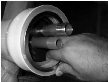
Removal of Retaining Ring
