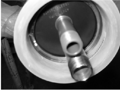
Retaining ring seated in the groove
