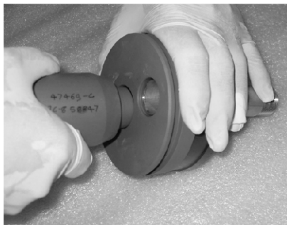
Removal of the Permeate port from the End Plug Assembly
