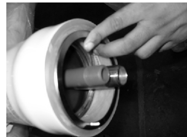
Inserting Retaining Ring into the groove
