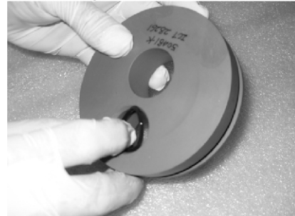
Inserting Permeate Port seal
