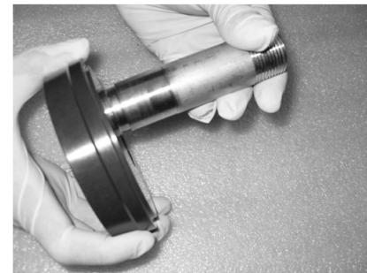
Removal of F/C Port from the Bearing Plate
