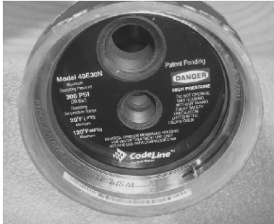
Retaining ring seated in the groove
