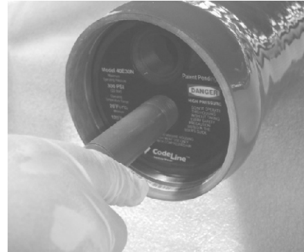
Removing the head assembly
