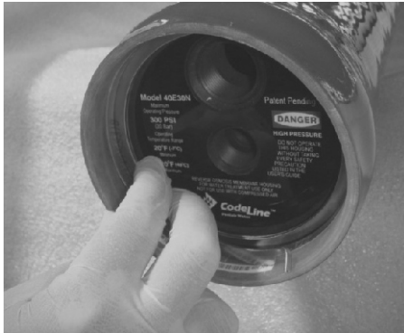
Removal of Retaining Ring
