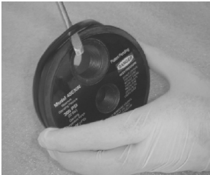
Removal of the Plug Seal
