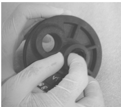
Inserting Adapter seal
