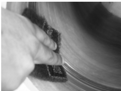
Cleaning inside the vessel
