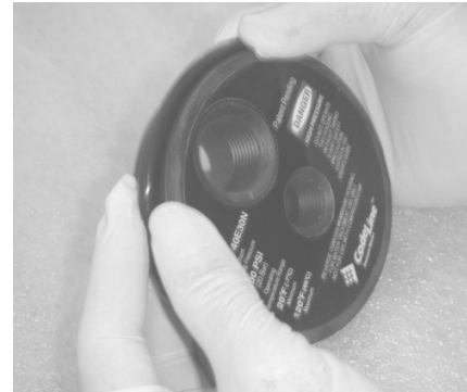
Inserting Head seal
