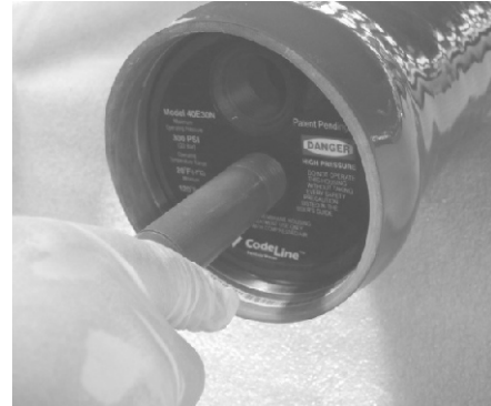
Installation of the End Plug Assembly into the vessel
