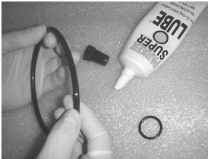
Lubricating Plug seals and O-rings
